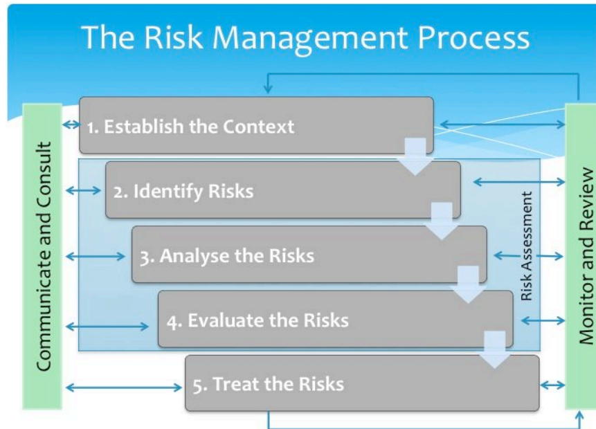
Figure 2: The 5 step risk assessment process used to identify priority areas for monitoring and surveillance/enforcement (adapted from AFMA 2013). Key to the success of this approach is input from key stakeholders in the identification and analysis of the risks and regular monitoring and review of the MCS protocol.
