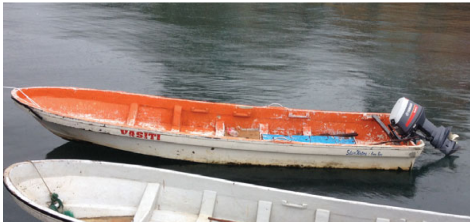
Figure 3. Typical fibreglass longboat (FRB) used by coastal fishermen in Fiji. Photo: D. Welch.
